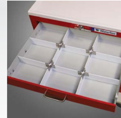
CUT & CLIP, FRONT TO BACK DIVIDER SYSTEM FOR STEEL CARTS Score the plastic strips and snap them to create your own divider system. Includes: (6) 22" long strips and 8 clips Additional clips available in a set of 6. (To fit into Steel Junior carts cut strips down to 16.5" long) DIV-CC2 (Dividers & Clips) DIV-CLIP (Clips)
